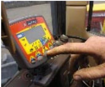
The Wizard of the ST model has a track marker and a metering shaft sensor for the seed axle as standard equipment.
