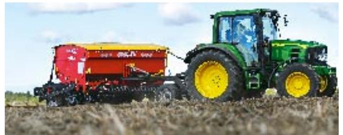
The seed hopper has mixing axles. The triangular bottom cones ensure that the hoppers empty evenly, even when you are seeding small seeds, such as rapeseed.
