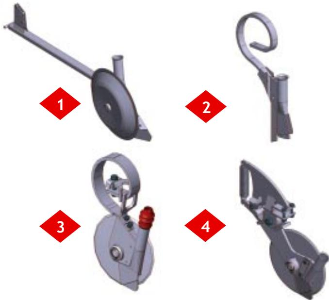
**1. The wedged disc coulters,** which is the seed coulters in all the machines. Keeps a good seeding depth, even under changing conditions. The rotating disc prevents the coulters from blocking. The side plate is easy to change.
