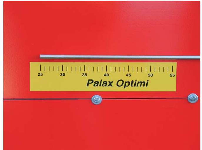
2. The stroke length can be optimised for 25...55 cm long billets
