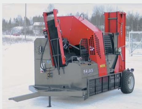
The machine can be towed by tractor using the special transport platform
