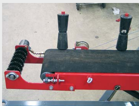
Hydraulic rear feed roller
